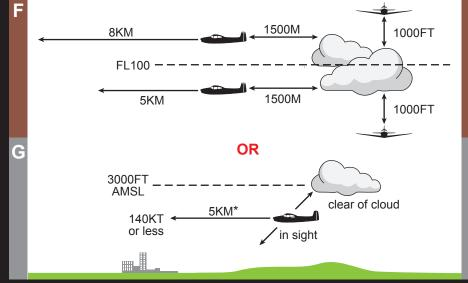
\* Aircraft (except helicopters) at 140KIAS or less: clear of cloud with the surface in sight in a flight visibility of at least 1500 metres. Helicopters at a speed which, having regard to the visibilty is reasonable: clear of cloud with the surface in sight in a flight visibilty of at least 1500 metres.
